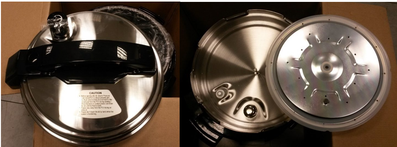
Figure 6 Lid upper and lower views; splash guard/seal carrier is removed from central mounting stud.
