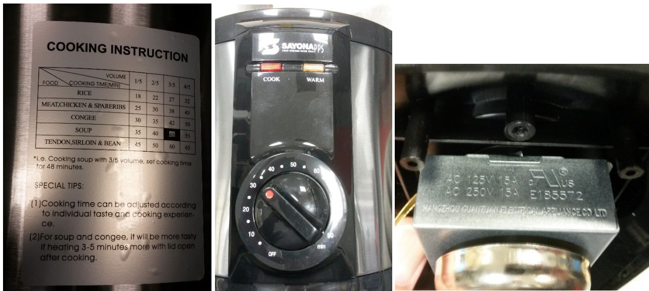
Figure 8 Cooking instruction label; rotary clockwork timer control knob and indicator lights; clockwork timer and bell.
