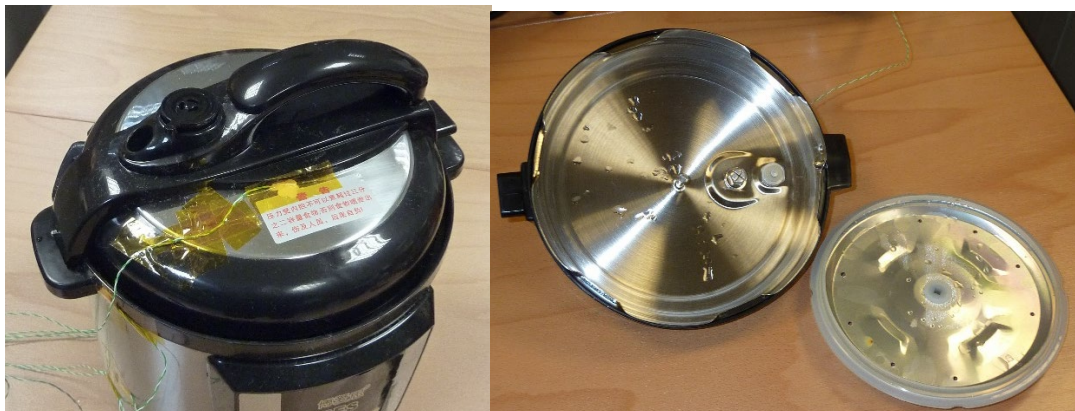
Figure 1. EPC and lid from above showing external thermocouple positions and from below with splashguard dismounted.
