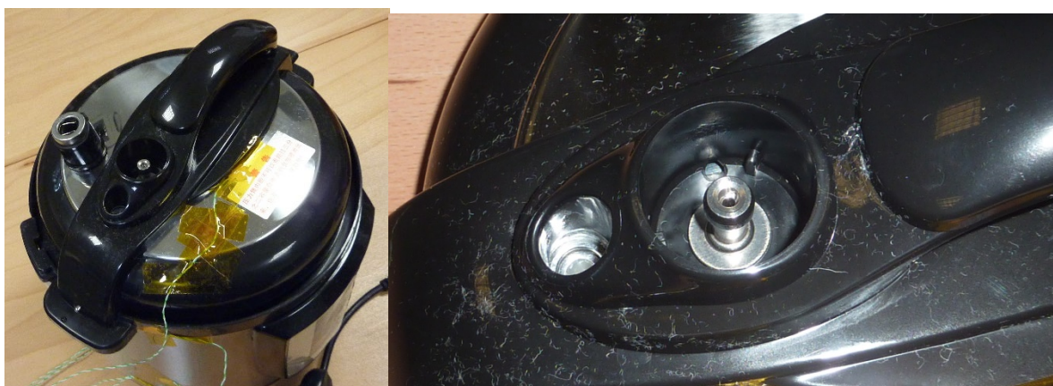
Figure 3. Top of BES 24 V DC EPC showing the weighted valve removed and close up of the orifice.
